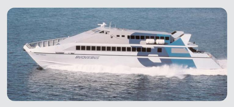
Sleek-lined and extremely fast, this catamaran ferry designed by Nigel Gee Associates and styled by Pininfarina is built by Derecktor to the highest quality standards with ABS, IMO HSC and USCG Sub H full compliance. It carries 300 passengers at a continuous-rating service speed of 53 knots
